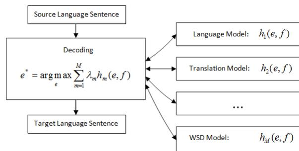
Figure 1: Architecture of Phrase-based Statistical Machine Translation
