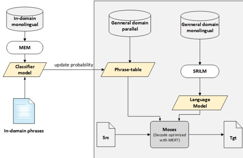
Figure 2: Architecture of the our translation model adaptation system
